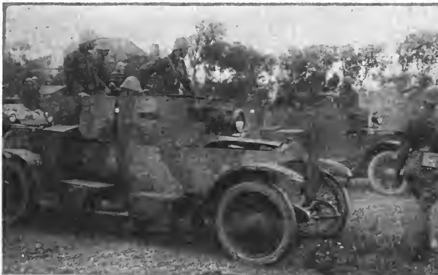
The Belgian armored cars in battle formation behind the lines. The cars differ in minor details such as the size and position of tool and ammunition box, etc. Note the steel-studded tires
